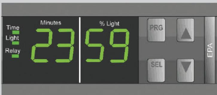
EPA Products Ltd has now introduced a digital dusk and dawn dimmer control. The digital dusk dawn control has been designed to be used with EPA high frequency energy saving fluorescent lighting, and tungsten lighting. Basic on/off times are still adjusted on a standard 24 hour lighting control clock. The first set of digits is the time span for lighting ramping up and down is adjusted from 1-99 minutes. The second set of digits is the desired brilliance adjusted as a percentage.
