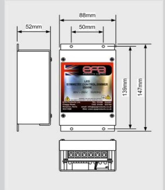
The EPA LED Symmetry control dimmer was designed with micro processor control to eliminate flicker associated with dimmable Led lights. Simple installation can be retro fitted to most lighting systems when upgrading to Led lighting. There is no requirement to install lighting filters / chokes or snubbers.
